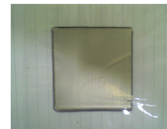
Fig 3 .Li deposition on polypropylene sheet.
